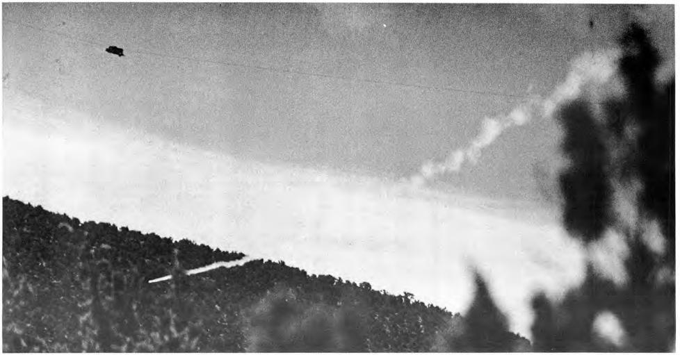
HEAT SEEKING Redeye missile veers away from the target carriage as it chases a decoy flare. Detector systems undergoing evaluation have sensed the missile
